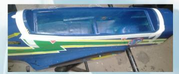
2-Sand the contact area at the canopy frame to improve glue adhesion. Clean up with a cloth.
