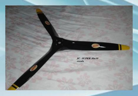
Three Blade 14x9 wood propeller, combustion engines
