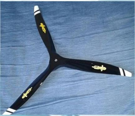
Three Blade 14x9 wood propeller, electric motors
