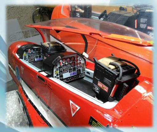
Custom made cockpit for T-27 Tucano 20cc, extremely detailed and realistic, ready to install in place of factory stock cockpit. Allows the installation of pilot busts (not full body).
