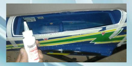
**3-**Apply the white glue in all the contact area. Clean up excessive glue with a cloth.
