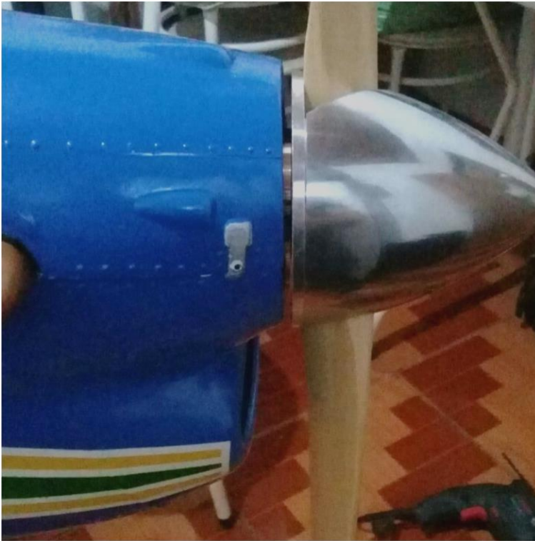
Above: parallel alignment between spinner/cowling (left) and engine axis/cowling (right).
