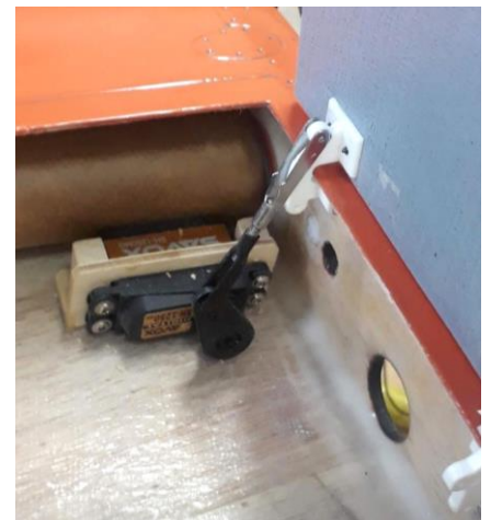
Above: door compartment hinges and micro servo installed with linkage.
