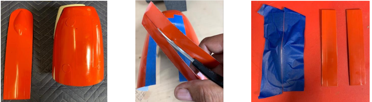
Above: Cutting process of the lower engine cowling and the 4 landing gear doors of the front landing gear.
