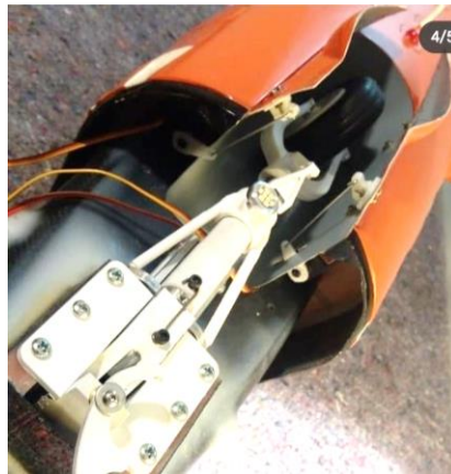
Above: left rear landing gear door servo of the front landing gear installed with linkage and horn (left), front landing gear position, rear doors, servos and horns (center) and 2 servos installed in the lower engine cowl for opening and closing the front landing gear doors of the front landing gear.
