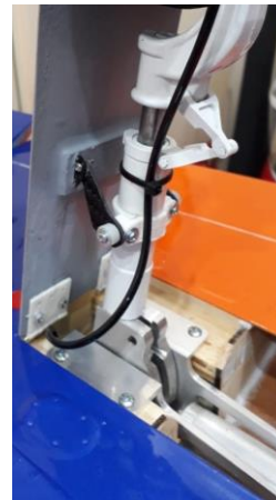
Above: detail of the articulated supports attachment to the external landing gear door of the external landing gear and closed external landing gear door (right).
