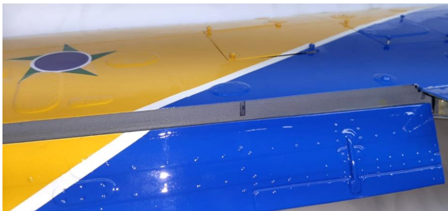
Above: gray areas (trailing edges) on ailerons and flaps shall not be drilled or cutted.
