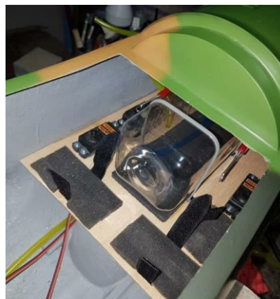
Above: Typical fuel tank position and throttle and choke servos position. Johnny Simões fuelers (right).
