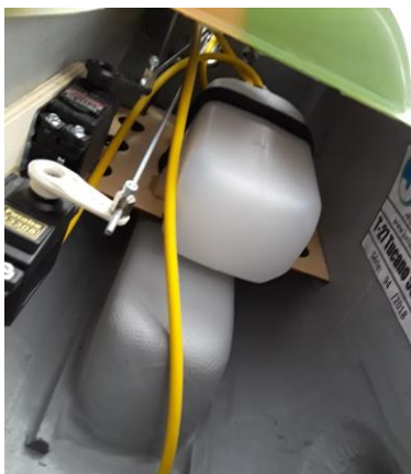
Above: Typical fuel tank position and throttle and choke servos position. Johnny Simões fuelers (right).
