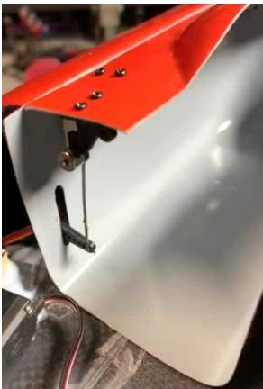
Above: left rear landing gear door servo of the front landing gear installed with linkage and horn (left), front landing gear position, rear doors, servos and horns (center) and 2 servos installed in the lower engine cowl for opening and closing the front landing gear doors of the front landing gear.
