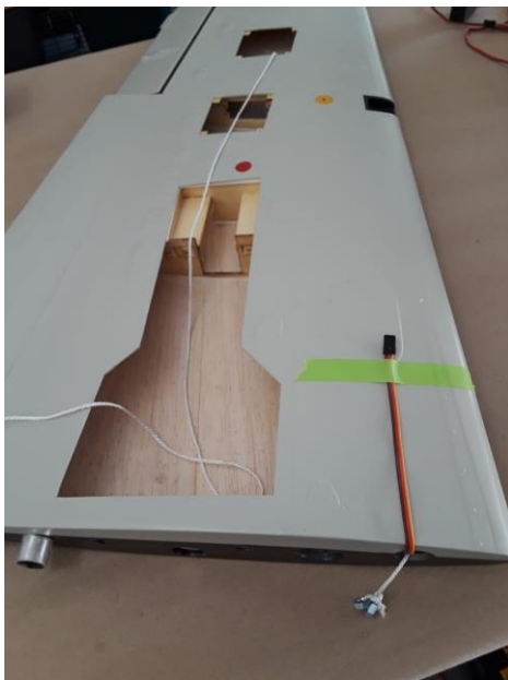
Above: thread and extensions passing process on wing (left) and connected and locked servos (right).
