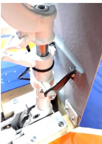
Above: detail of the articulated supports fixation to the external landing gear door of the main landing gear (left) and internal door of the main landing gear with opening and closing by pneumatic cylinder (right).
