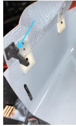
Above: the 2 rear landing gear doors of the front landing gear in the final position (left), the horn installed in the rear door of the front landing gear (center) and the place of attachment of the micro servo (right).
