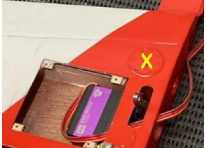
Above: Position of the tube in the middle of the stabilizer and fuselage (left) and detail of the hole location (indicated with the yellow letter X) for fixing the stabilizer halves in the stabilizer tube (right).
