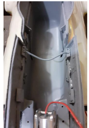
Above: installation of a mechanism for opening and closing the doors of the front landing gear.
