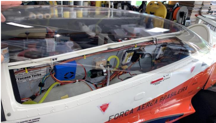
Above: clear canopy cutted and ready to glue (left) and glued and in place with masking tape.
