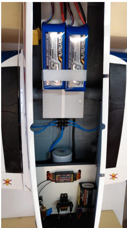
Above: Li-Po batteries used in electric motorization. Final position to be defined after correct C.G. balance.
