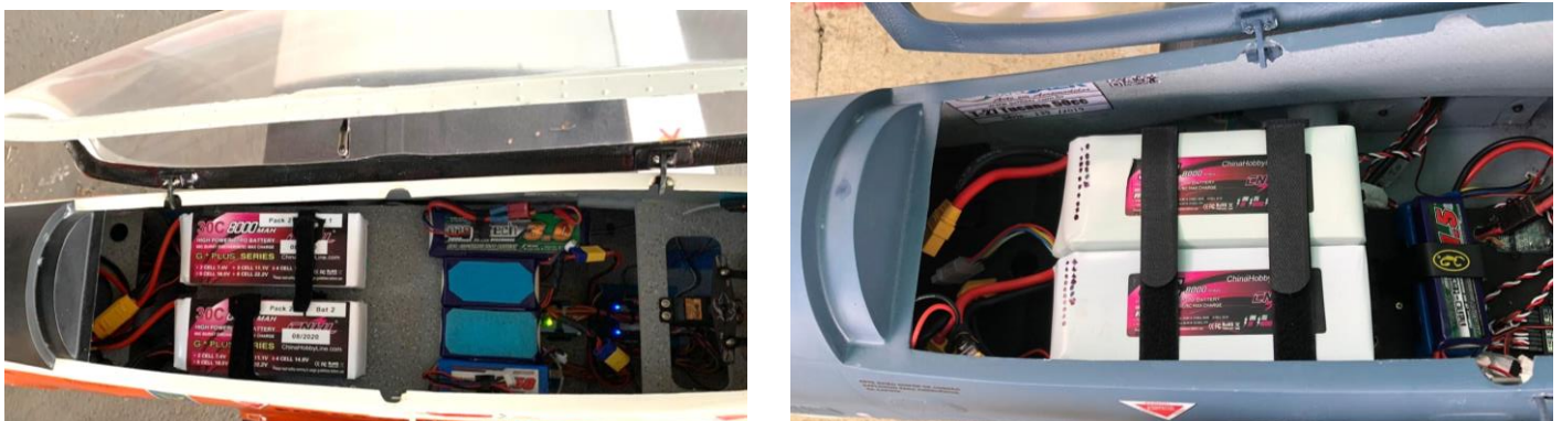
Above: equipment installation examples in the fuselage interior on electric motor version and Li-Po batteries position.
