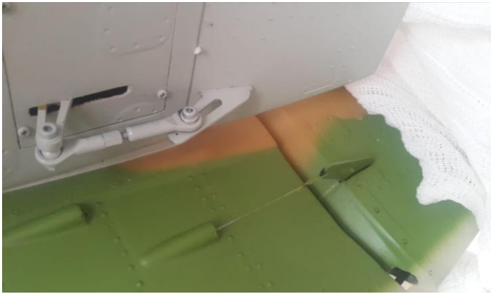
Above: elevator servo, servo arms and horns position and pull-pull steel cables exits with rudder double horn.
