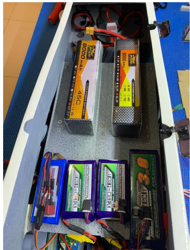
Above: Li-Po batteries used in electric motorization. Final position to be defined after correct C.G. balance.
