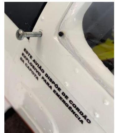
Above: Screws to ensure total security when attaching the canopy and canopy frame.
