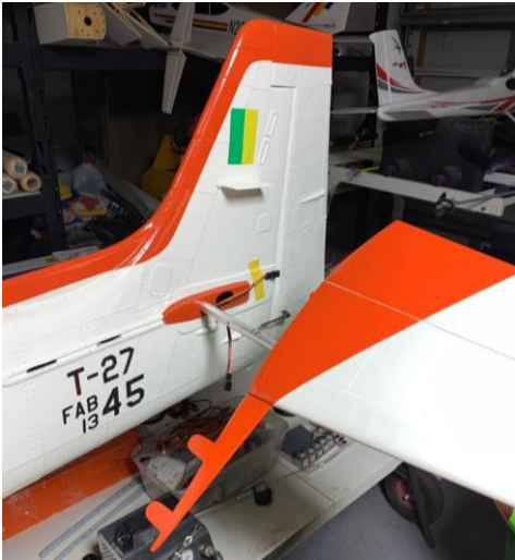
Above: Position of the tube in the middle of the stabilizer and fuselage (left) and detail of the hole location (indicated with the yellow letter X) for fixing the stabilizer halves in the stabilizer tube (right).
