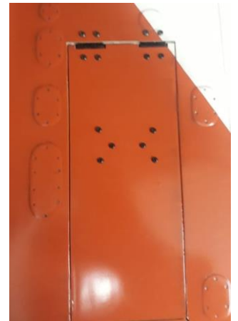
Above: detail of the articulated supports attachment to the external landing gear door of the external landing gear and closed external landing gear door (right).
