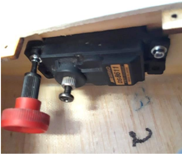
Above: Short screwdriver and correct position to screw the wing's servos.
