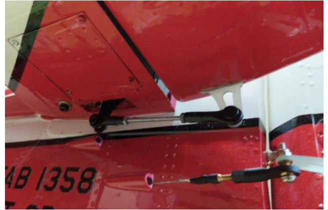
Above: elevator servo, servo arms and horns position and pull-pull steel cables exits with rudder double horn.
