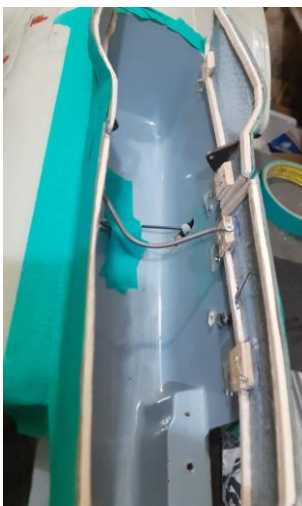
Above: installation of a mechanism for opening and closing the doors of the front landing gear.
