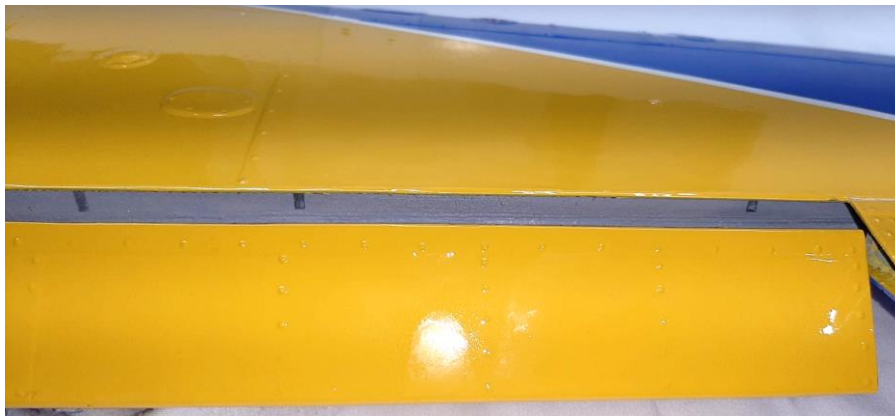
Above: gray areas (trailing edges) on stabilizer shall not be drilled or cutted.
