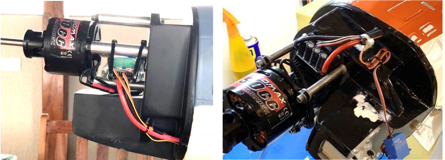
Above: electric motor installation and speed control on horizontal position (left) and vertical (right).
