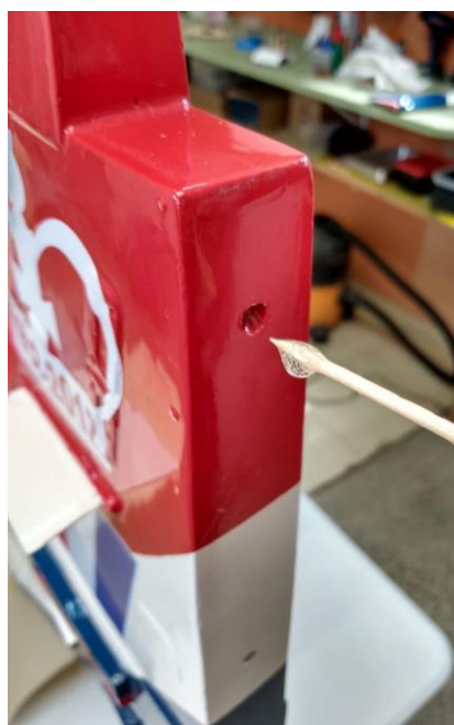
Above: rudder hinge points epoxy gluing sequence.
