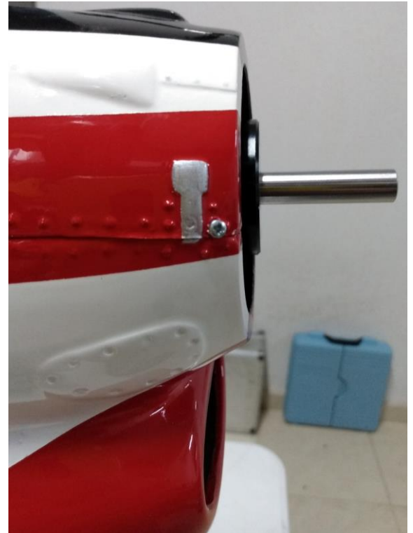
Above: parallel alignment between spinner/cowling (left) and engine axis/cowling (right).
