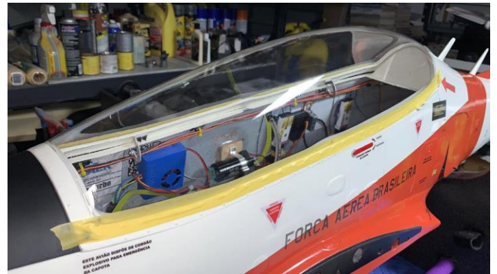
Above: clear canopy cutted and ready to glue (left) and glued and in place with masking tape.
