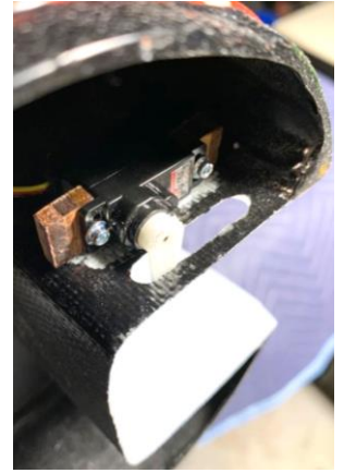
Above: the 2 rear landing gear doors of the front landing gear in the final position (left), the horn installed in the rear door of the front landing gear (center) and the place of attachment of the micro servo (right).
