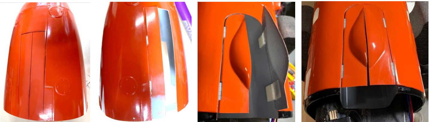
Above: fixed with Dubro hinges, the two front landing gear doors of the front landing gear in the lower engine cowling (left) and the two rear doors of the front landing gear in the fuselage (right).
