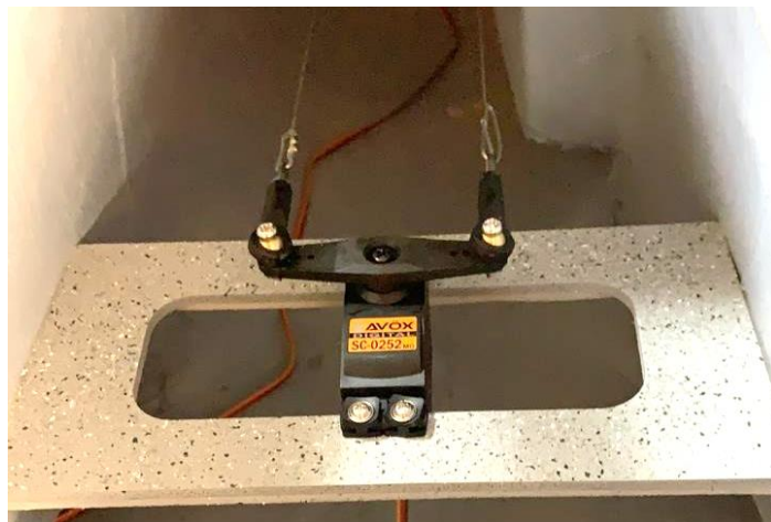
Above: rudder double horn (left) and rudder servo position on tray inside the fuselage (right).
