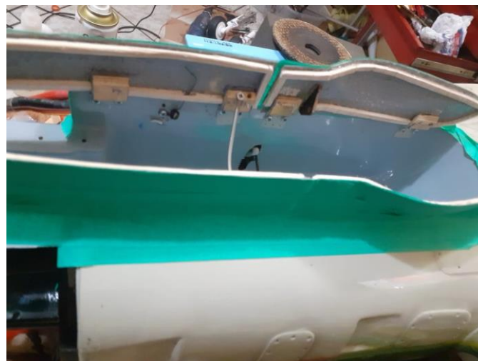
Above: installation of a mechanism for opening and closing the doors of the front landing gear.
