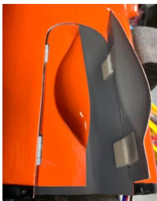
Above: fixed with Dubro hinges, the two front landing gear doors of the front landing gear in the lower engine cowling (left) and the two rear doors of the front landing gear in the fuselage (right).
