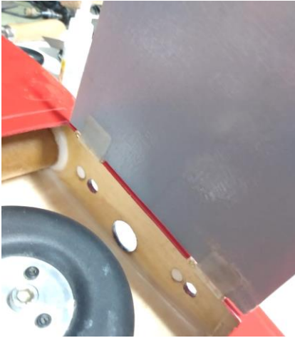
Above: Dubro hinges installed on internal landing gear doors.
