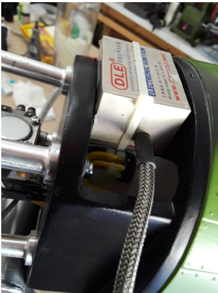
Above: ignition module installation behind the firewall on upper side (left) and lower (right).
