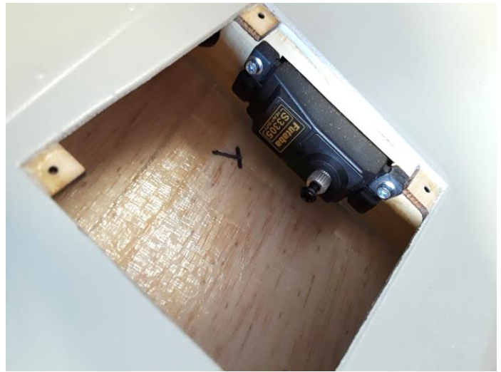
Above: Short screwdriver and correct position to screw the wing's servos.
