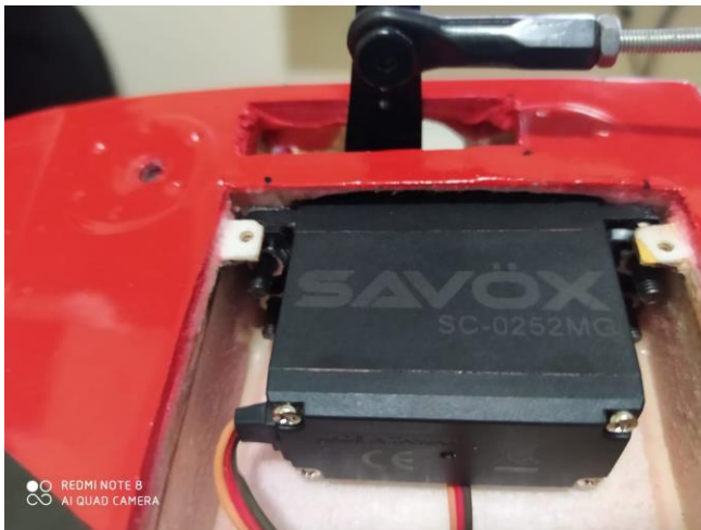
Above: elevators servos, servo arms and horns position.
