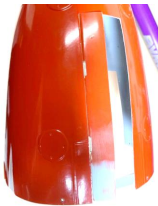
Above: fixed with Dubro hinges, the two front landing gear doors of the front landing gear in the lower engine cowling (left) and the two rear doors of the front landing gear in the fuselage (right).
