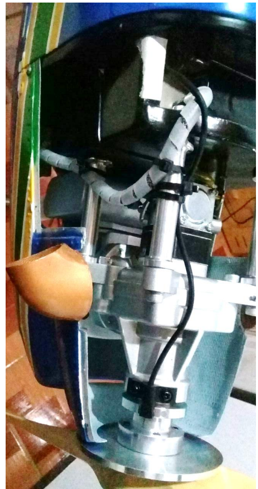
Above: ignition module installation behind the firewall on upper side (left) and lower (right).
